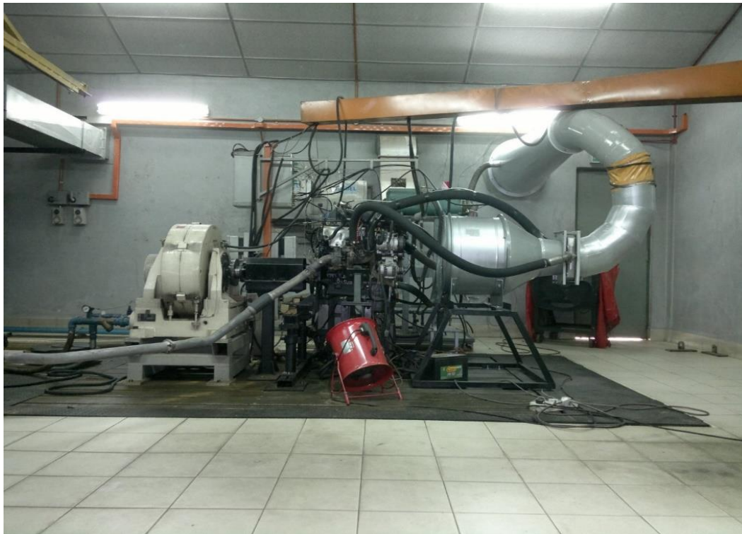
Fig. B Modified layout with the addition of cooling system to turbo-intercooler.
