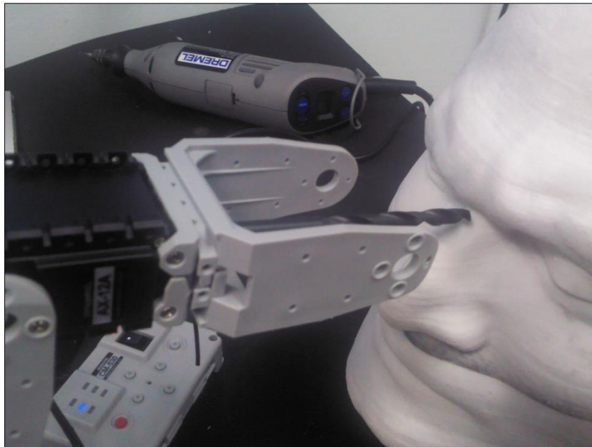
Figure 6.4: A photograph of the 3D mock operating room setup being used to perform image-guided navigation with the artificial patient.
