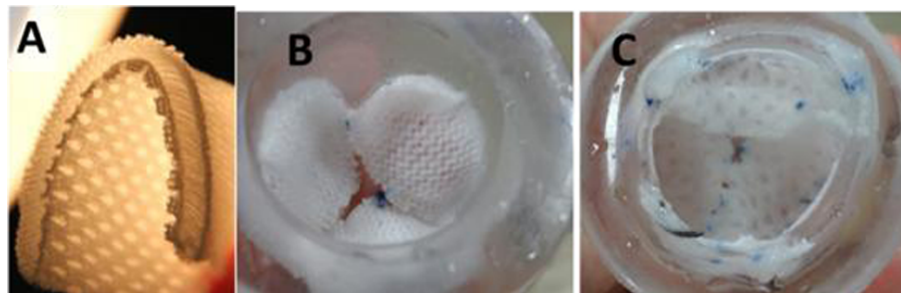
Figure 17. Three-dimensional weft-knitted spacer fabric made out of PET yarn, originally made for sport-garment.
