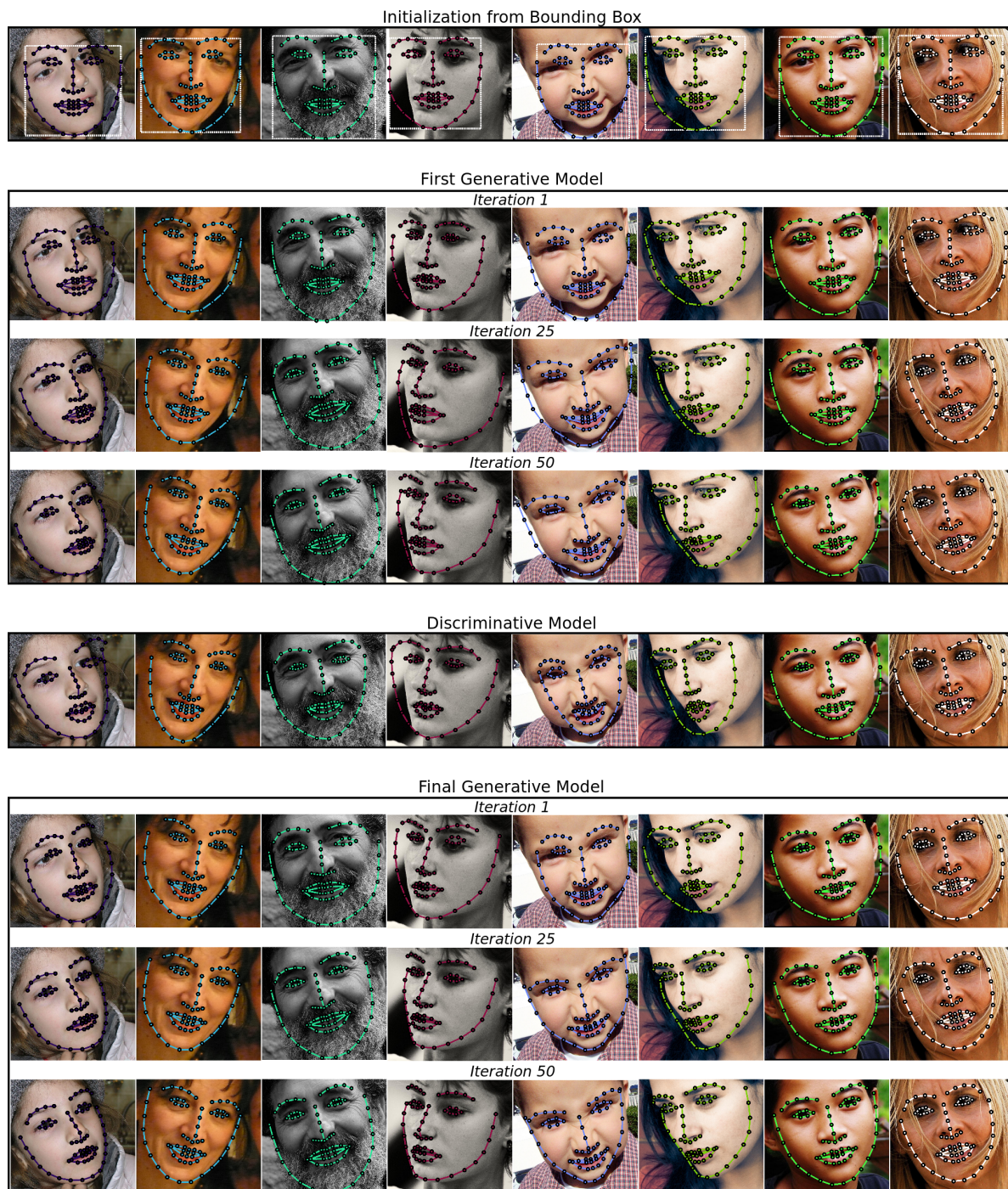
Figure 6.8: Automatic construction of AAM with a single application of the discriminative model. The figures show the evolution of the fitted shapes for 8 images, starting from the bounding boxes. Each automatically trained generative model is performed for 50 iterations.
