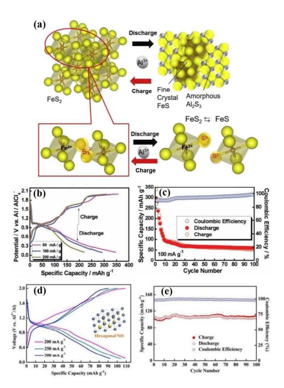
**Figure 6** (a) Schematic charge-discharge reaction model of FeS<sub>2</sub> with aluminum ions at 55 °C, Reprinted with permission from Ref. [31], Copyright 2016, Elsevier Publishers (b) The charge/discharge curves of Ni<sub>3</sub>S<sub>2</sub>/Graphene cell for the second cycle at the current densities
