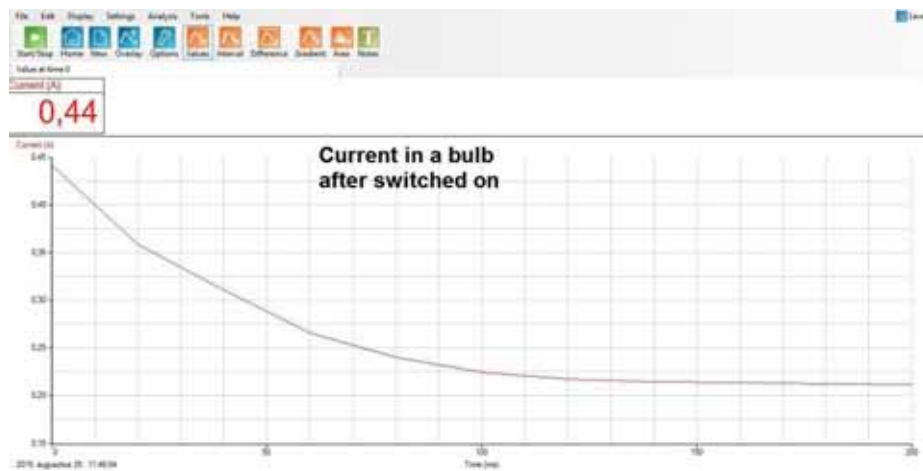
Fig.4. Current falls according to the increasing resistance [3]
