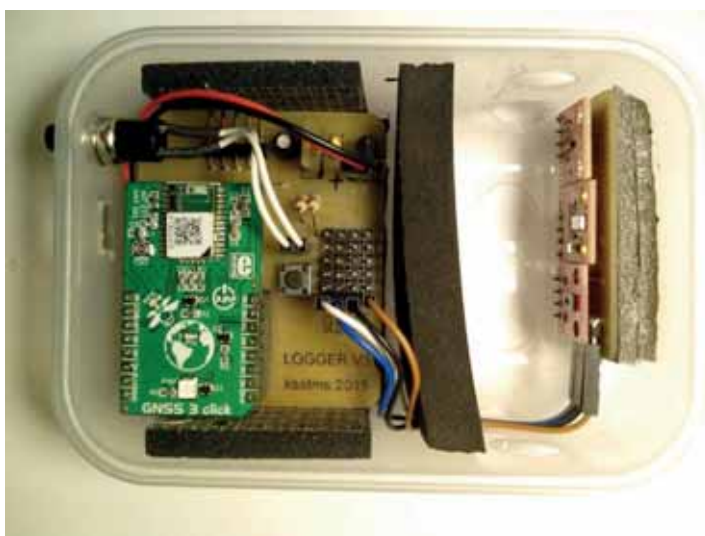
Fig.2. The measuring module housed in a plastic box - data logger with GNSS click (left) and the set of sensors (right)
