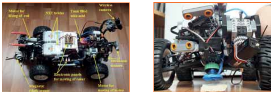
Fig.6. The Husar-5 rover with the Carbonate experiment instruments [20]
