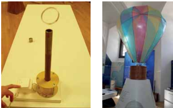
Fig.3. Left panel: The Lenz cannon. Right panel: The hot air balloon is ready to start
