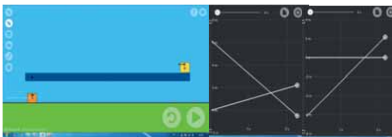
Fig.8. The effect of changing the reference system. The displacement-time graph on the left is measured from a stationary reference system, while the graph on the right is measured from a system fixed to the yellow box
