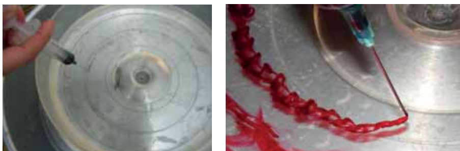
Fig.6. Left panel: rotating disc with cylindrical vessel with water, Right panel: von Kármán vortex street visible behind the syringe
