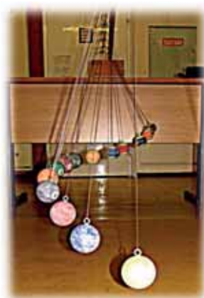
Fig.1. Snapshot of a pendulum wave (front view)
