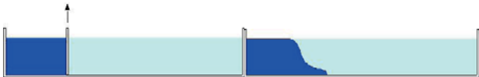
Fig.4. Left panel: Water tank separated in two by a glass with cold water in the left and warm in the right. Right panel: After removing the separator, the cold water moves similarly with the cold front [7]
