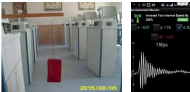
Fig.7. Acceleration-time graph of the damped oscillation
