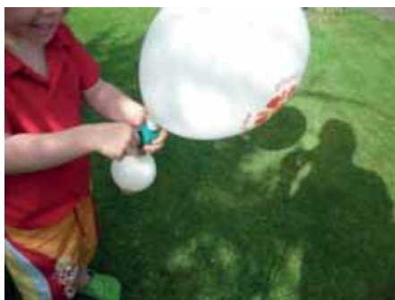
Fig.4. Large and small balloons. When joined the smaller balloon inflated the larger one.
