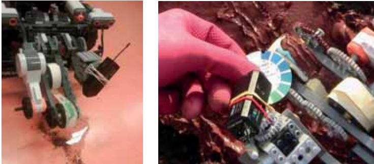
Fig.3. On the front of the rover there is an ultrasonic sensor of the obstacles before the rover. (Upper arm). There is also the camera (right up) and there is the arm moving the indicator ribbon. The ribbon is rolled from one wheel to the other wheel while the arm is contacting the surface and soil. The camera observes the changes on the indicator ribbon colour [18]
