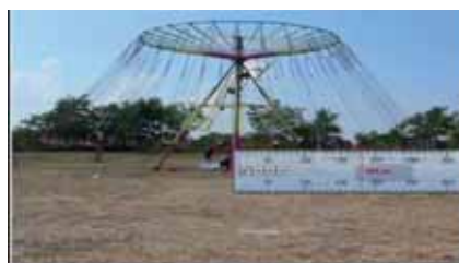
Fig.7. The \alpha angle can be measured with a goniometer, the radius with a pixel bar
