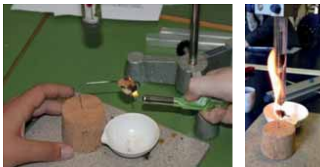
Fig.2. Left panel: the experimental apparatus for evaluating the calories of foods made in the science lab, where a student was starting the combustion. Right panel: the apparatus during the combustion.
