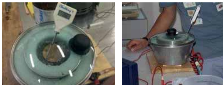
Fig.4. Left panel: Prototype of the modified bomb calorimeter showing the flow of air bubbles in the water. Right panel: the apparatus used by students for a measurement.
