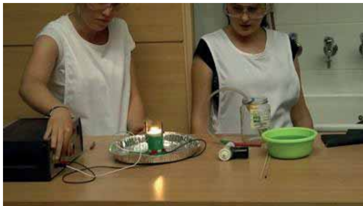
Fig.6. The pencil refill starts glowing dazzlingly because of the Joule heat. The reaction between the carbon and the oxygen increases temperature
