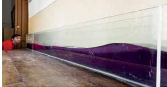
Fig.3. Soliton wave in a water tank, after the removal of the separator, presented at the Saturday of experiments event in 2015
