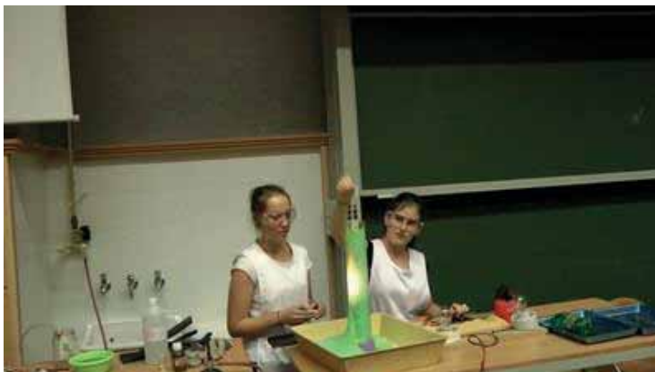
Fig.4. A burning match began to glow dazzlingly because of the oxygen.
