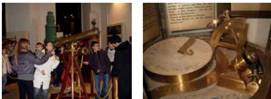
Fig.5. Left panel: Reflecting and refracting telescopes in the Astronomical Museum. Right panel: The sundial cannon, it can indicate noontime by a cannon-shot
