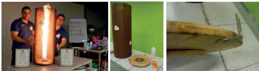
Fig.3. The self-developed fire tornado and the equipment
