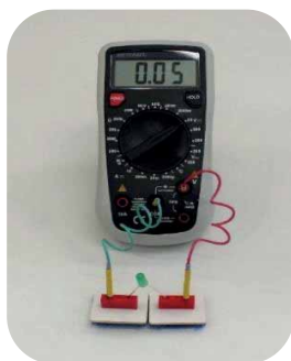
Fig.11. The LED's voltage is rather low in room light
