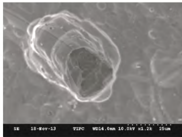
(b) conventional SEM image over-corrosion spot(×300)
