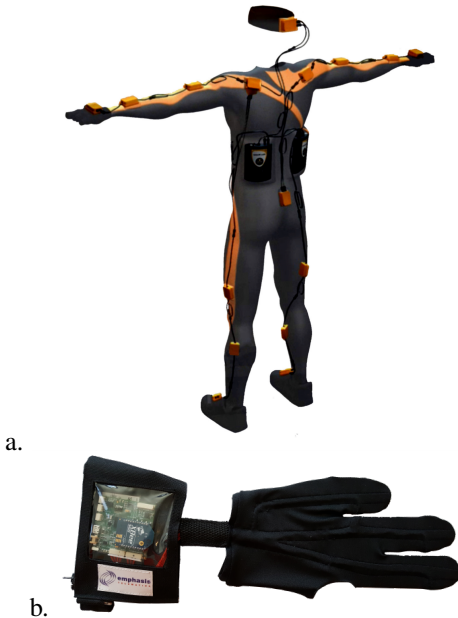
Figure 1. Wearable sensors used in the experiment: (a) XSens MVN suit [16]; (b) e-glove from Emphasis Telematics.
