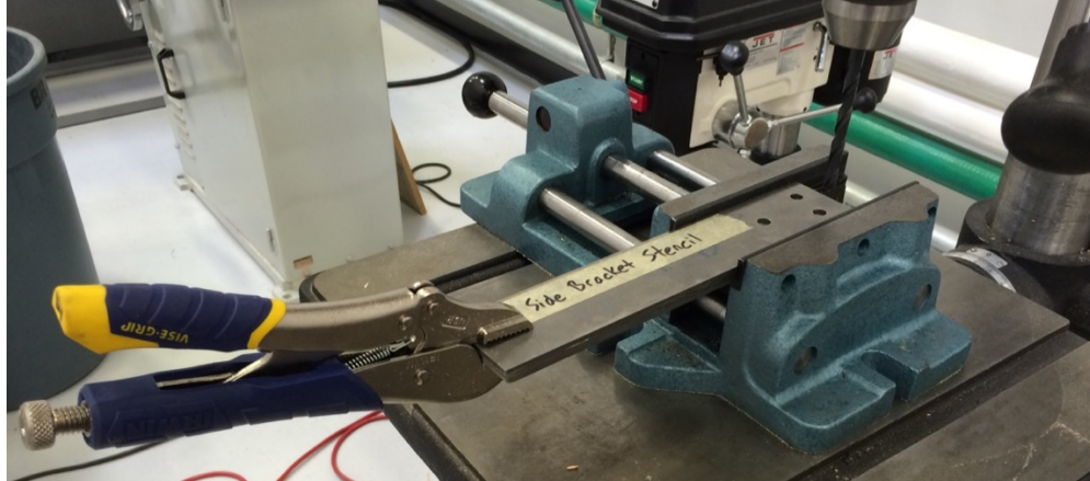
Figure 27: Side Brackets and Stencil in the Drill Press Vise
