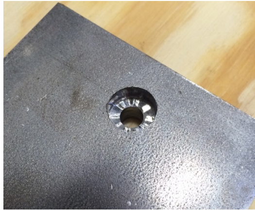
Figure 7: Pocket and Through-Hole in Prototype Side Bracket
