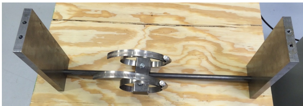
Figure 12: Slider Subassembly Sitting Upside Down
