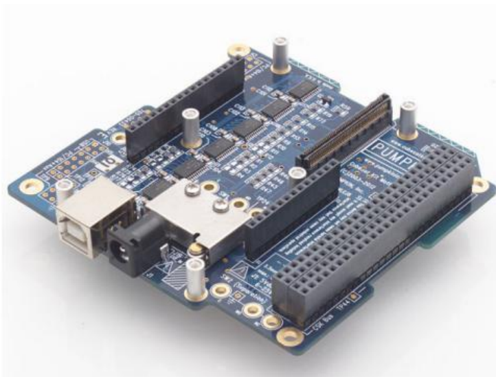
Figure 2.2.1: A single board computer motherboard for harsh environments.
