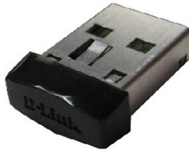
*Fig. 20: Microadaptador Wireless USB D-Link [Dli,www].*
