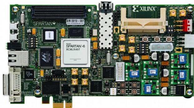
*Fig. 11: Xilinx Spartan-6 FPGA Embedded Kit [Xil, www].*
