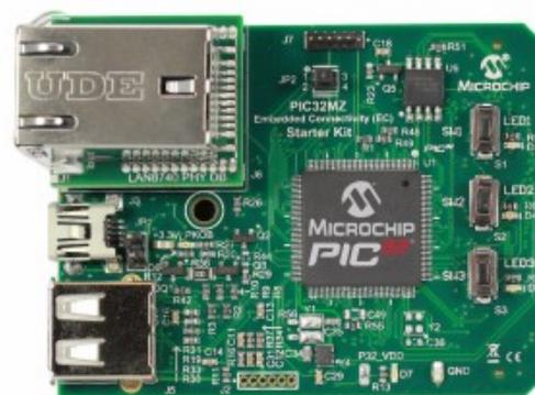
Fig. 10: PIC32MZ EC Starter Kit [Mic,www].
