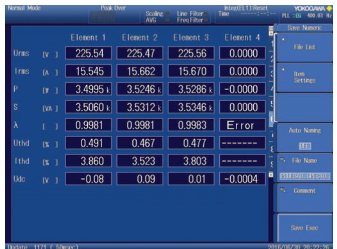
Figure 11. Input power quality at 400 Hz without L_g
