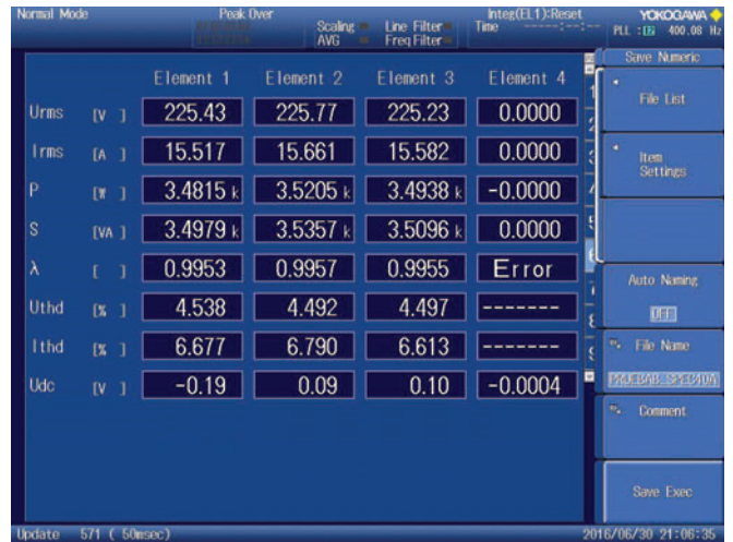
Figure 9. Input power quality at 400 Hz with L_g = 300 \mu\text{H}
