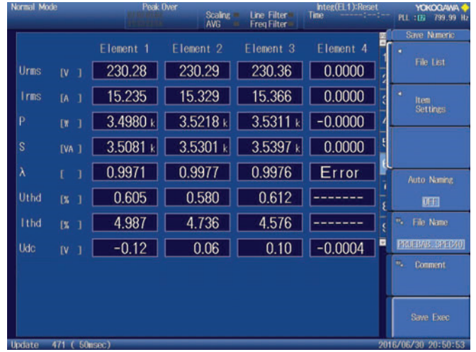
Figure 15. Input power quality at 800 Hz without L_g
