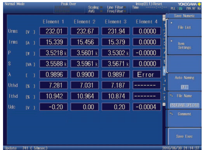
Figure 10. Input power quality at 800 Hz with L_g = 300 \mu\text{H}
