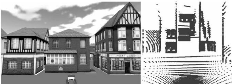
Fig. 3. 3D collision points. Representation of what the 3D laser is scanning at a given moment.
