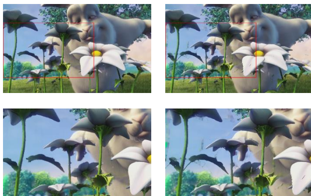
Figure 11. Globally optimized view synthesis (left) vs. VSRS (right)
