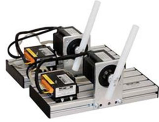
Fig. 7. 1DoF master-slave-system (courtesy of sensodrive)
