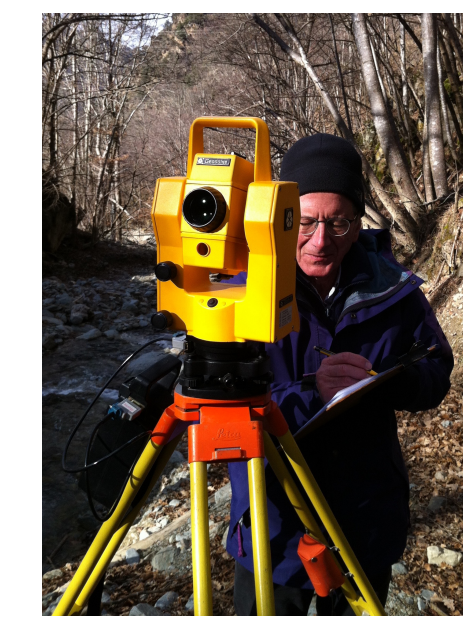
Figure 4: Theodolite measurements were conducted using the Geodolite 502 Total Station, which has an angular precision of 6'' and a distance accuracy of ±5mm+5ppm.
