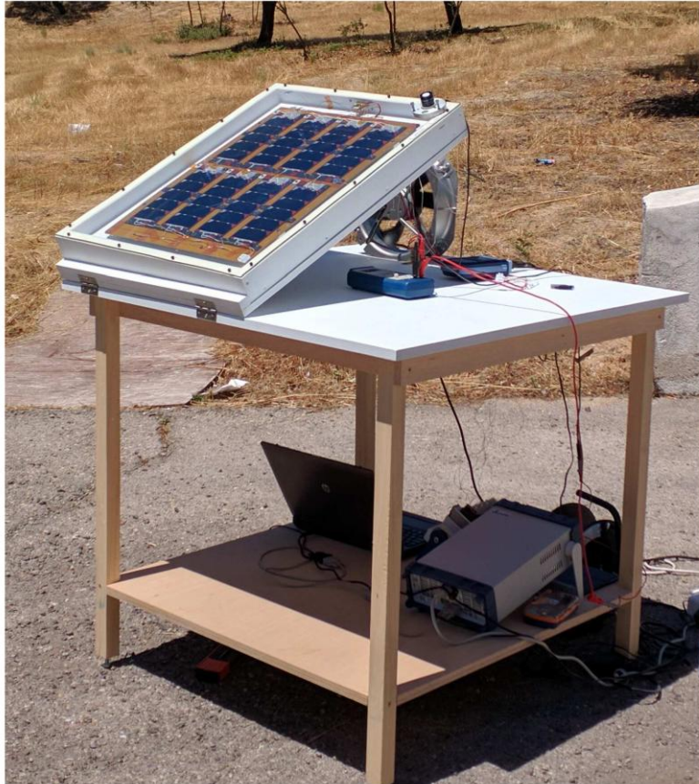
Figure 10. Testing Sep-up for the UPMSat-2 Solar Panels
