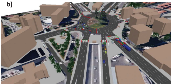
Fig1. Real traffic network image from FL (a) vs. simulated network with the VISSIM model (b)
