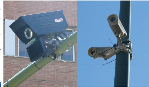
Fig2. Video cameras deployed to characterize traffic fluxes composition and detailed routes
