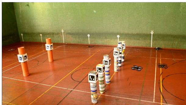
Fig. 1. Experimental flight of the basic instance of the framework, which is characterized by swarm behavior, using 5 AR Drones. The row of columns represents a virtual wall with a single 1.5 m opening in the middle. In order to simplify the localization problems the columns are marked using ArUco visual markers [2]. In this flight the mission of the swarm is to cross from one side to the other, each swarm agent also has to avoid collision with the columns or the other drones. This test was designed to showcase the capabilities of the basic instance of the framework.
