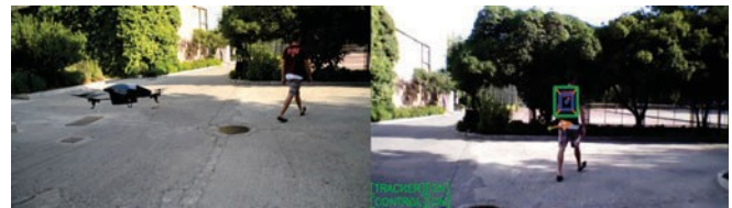
Fig. 1. (left) Image of the AR Drone 2.0 during one of the object tracking and following experiments. The drone is equipped with the outdoors hull to improve the system's wind disturbance rejection.
