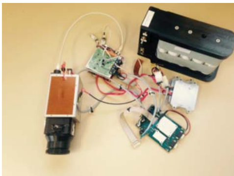
Figure 3: Some IR camera devices (current converter, SSD, IR camera module and the electronic).
