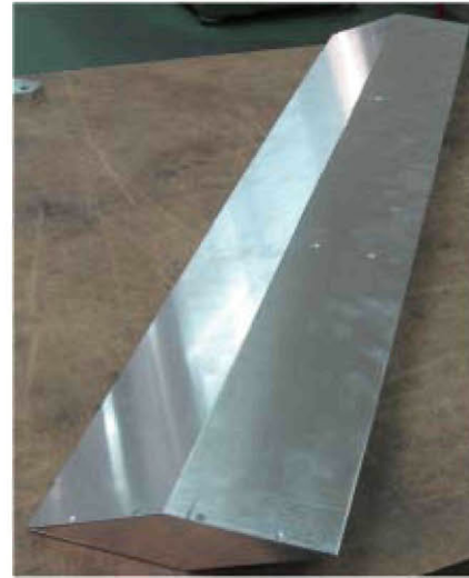
Fig. 10 Prototype: ideal PEC rhombic cross section strut of L=216.8\text{ mm} and W=54.2\text{ mm}
