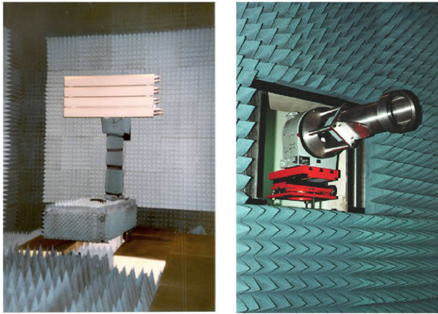
Figure 3: UPM, Spherical Near-Field Antenna Test Facility. AUT Positioner on longitudinal table and Roll over Azimuth Polarization Positioner.
