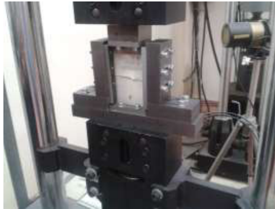
Figure 4. Airbus AITM-0010 compression tool after impact
