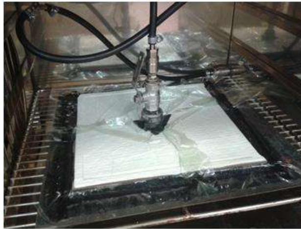
Figure 3. Panel ready for curing
