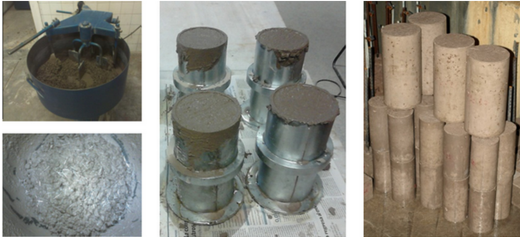
Fig. 2. Manufacture and curing of cylindrical specimens with and without addition.
