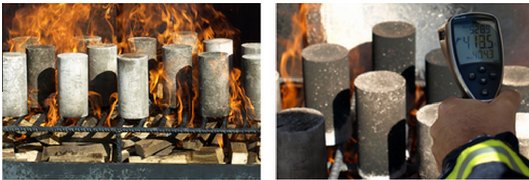
Fig. 3. Fire test with direct exposure to the flames of the specimen surface, and measurement with infrared thermometer.
