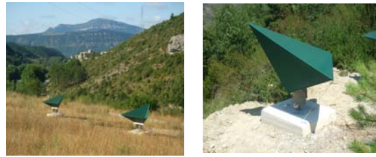
Figure 13. Corner reflectors installed in Itoiz.
