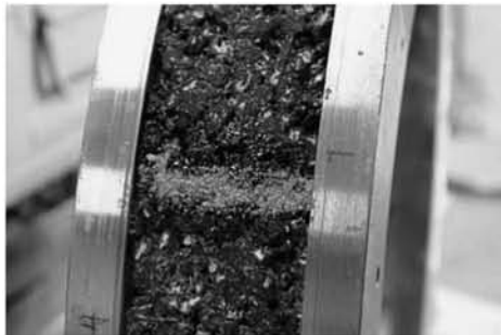
Fig. 8. Detail of the protective seal placed at the joints between the specimens.
