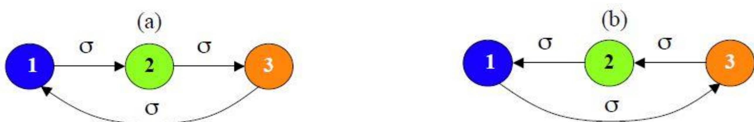
Figure 1: Ring configurations of three oscillators unidirectional coupled in (a) forward and (b) backward directions.
