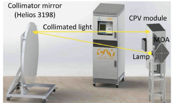
Fig. 4. (Color online) Scheme of the solar simulator for CPV modules Helios 3198. A xenon lamp is placed at the focus of the collimator mirror to measure the electrical properties of modules (while the module is illuminated with collimated light). The module optical analyzer is installed at the focus of the collimator mirror to characterize the optical-angular properties of CPV modules (while the module is emitting light).
