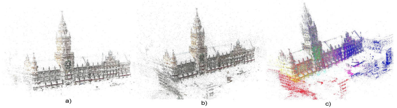
Fig. 4. a) Base point cloud model, and b) Bundler’s final model vs. c) ours, in which colors map different videos.
