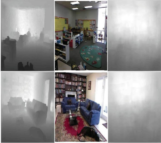
Fig. 4. From left to right: ground truth depth, query image and depth estimate computed by the proposed algorithm.
