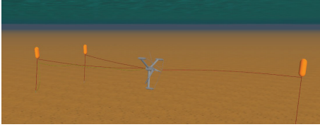
FIGURE 2: Mooring system based on wires and buoys.
