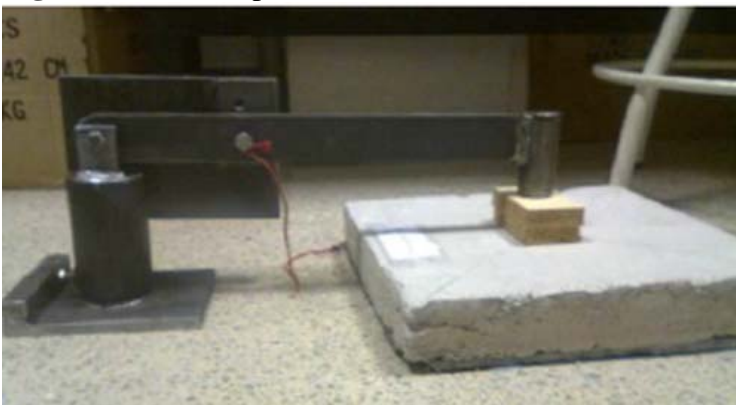
Figure 2. Hammer placed and levelled on o wood blocks.
