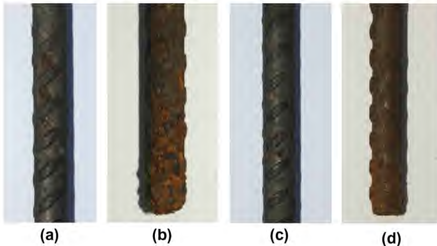
Fig. 5. Symptoms of corrosion in the rebars embedded in the mortar specimens, with the following characteristics: (a) LFS and 0.4% \text{Cl}^- , (b) LFS and 2.0% \text{Cl}^- , (c) reference specimen with 0.4% \text{Cl}^- and (d) reference specimen with 2.0% \text{Cl}^- .
