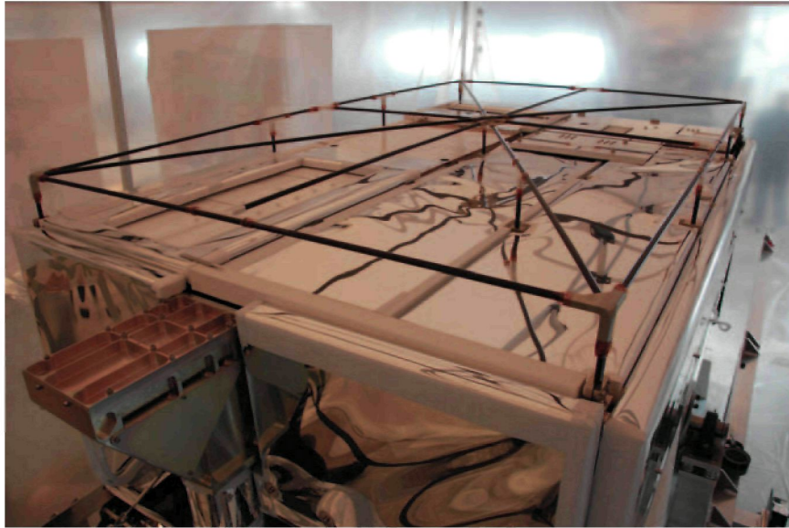
Fig. 6 PFI platform sitting on SUNRISE telescope before setting the protective wind shield
