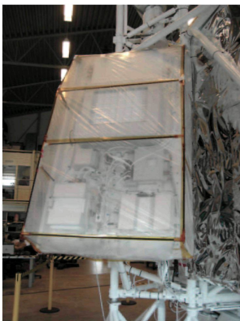
Fig. 5 PFI electronics rack with the wind shield
