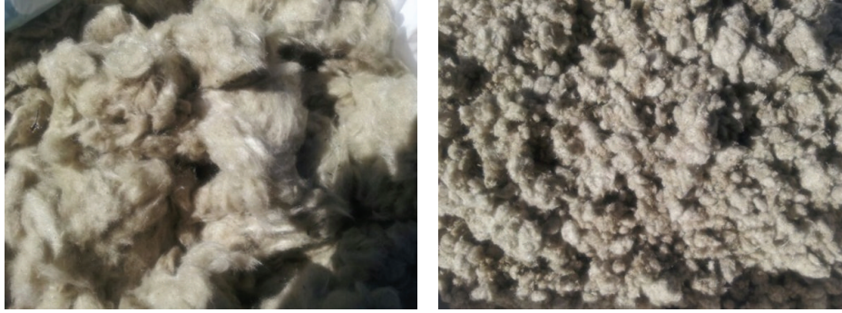
FIGURE 3: Rock wool recycling before and after being processed.
