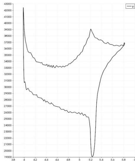
Figure 17 Absolute pressure distribution, profile 1/3 height, t=0.1 s, U_{\infty}=240 m/s, 10 9 conventional rudder, 3D
