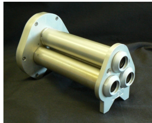
FIGURE 2. Tri-band spectroheliometer based in isotype cells
