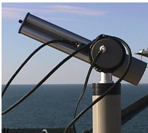
FIGURE 1. CIMEL Photometer, the instrument used by the AERONET network
