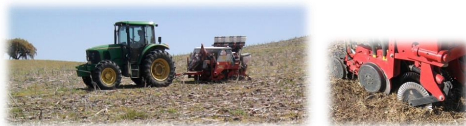
Figure 1. Double disc furrow opener vacuum seeder and tractor during the sowing operation and side gauge wheel depth control.
