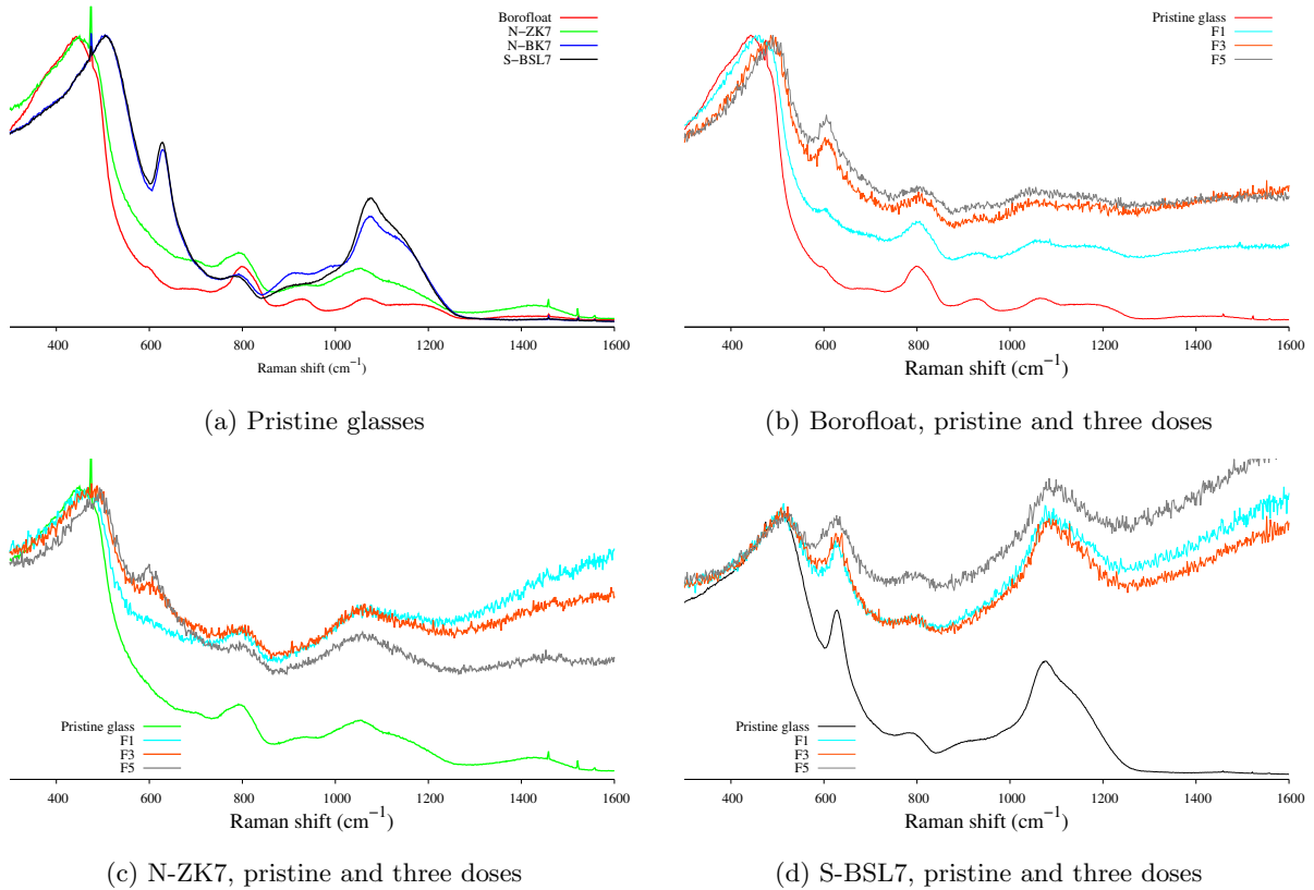
Figure 1: Raman spectra of the glasses, irradiated and non irradiated samples . (a) Pristine glasses, (b) Borofloat, (c) N-ZK7, (d) S-BSL7
