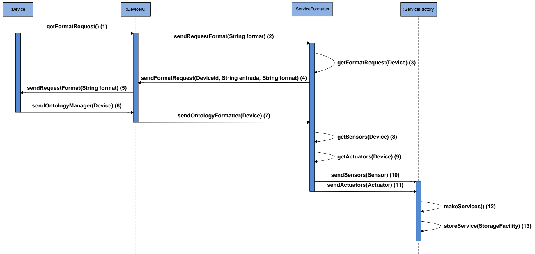
Figure 25. Registration sequence diagram
