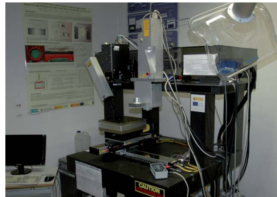
Figure 5: Laser station for LIFT processes at UPM.
