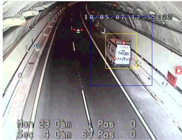
Fig. 3. Stopped Vehicle Detection at the entrance of a tunnel of M-12 toll road in Madrid (Spain)
