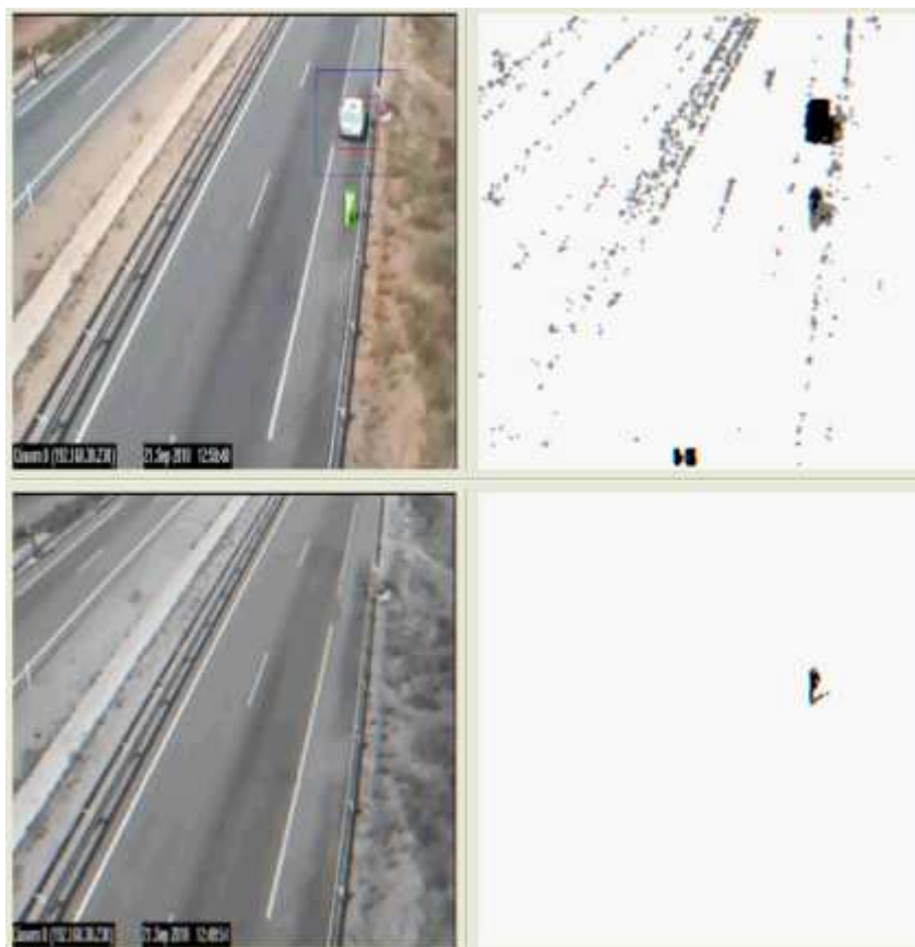
Fig. 2. Stopped vehicle and driver detection in a Spanish highway. From left to right, up to down, different results can be visualised: final result offered to the operator in the control centre of the highway, transience map, modelled background and pedestrian detection.
