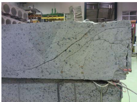
Figure 21. Vertical section of sawn slab
