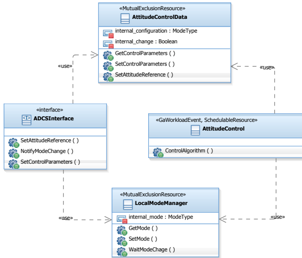
Fig. 4. Detail of the ADCS subsystem UML class diagram
