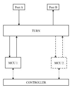
Fig. 3: Single allocation configuration.
