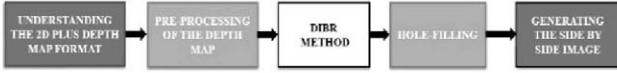
Figure 2. Functional Flow Block Diagram of the module of generation of synthetic views
