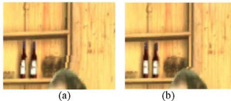
Figure 9. Magnified images of a certain region of the synthetic images after: (a) asymmetric Gaussian filter; (b) edge dependent filter.
