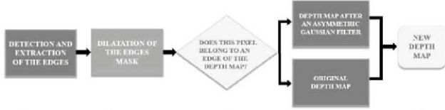
Figure 5. Functional Flow Block Diagram of the edge dependent filter
