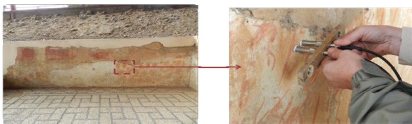
Fig. 4. UPV measurements on SDH13MA wall from Mitreo’s House (Photo by Natalia Perez)
