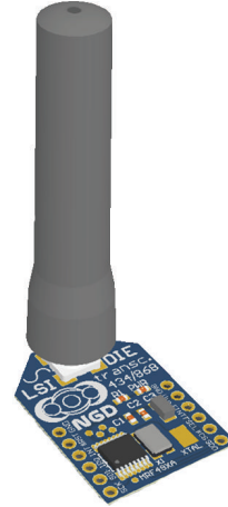
FIGURE 3: A 3D model of the implemented MRF49XA RF module.
