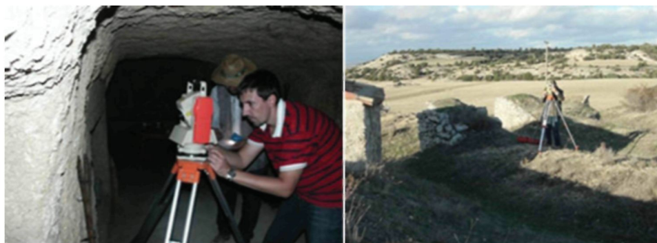
5 Topographic mapping with Pentax R-325N Total Station
